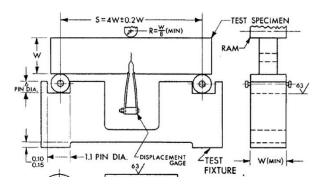
Fig. 7. Bend test fixture design (ASTM 399).
