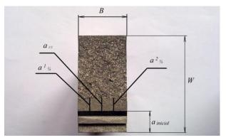
Fig. 13. One specimen after breaking
