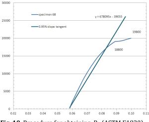
Fig. 10. Procedure for obtaining  $P_Q$  (ASTM E1820)
