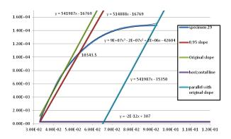
Fig. 12. Procedure for *J* calculation (ASTM E1820).
