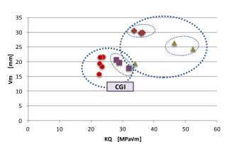
Fig. 14. Fracture Toughness of SGI and CGI in terms of  $K_Q$  [MPa $\sqrt{m}$ ] and  $V_m$  [mm].
