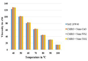
Fig. 7 Viscosity (cSt) of Lubricating oils.
