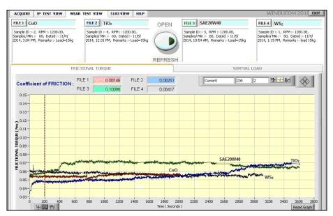
Fig. 3. Friction torque for various lubricating oils.
