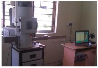
Fig. 1. Four ball tribometer.
