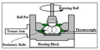
Fig. 2. Schematic diagram of Four ball tribometer.
