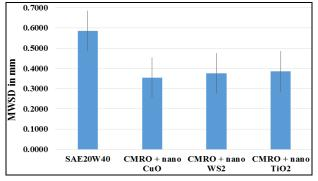
Fig. 5. Mean wear scar diameter of lubricating oils.
