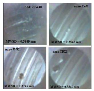
**Fig. 6.** Wear scar image of lubricating oils (Magnification 50X).
