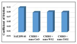
Fig. 4. Coefficient of friction for various lubricating oils.
