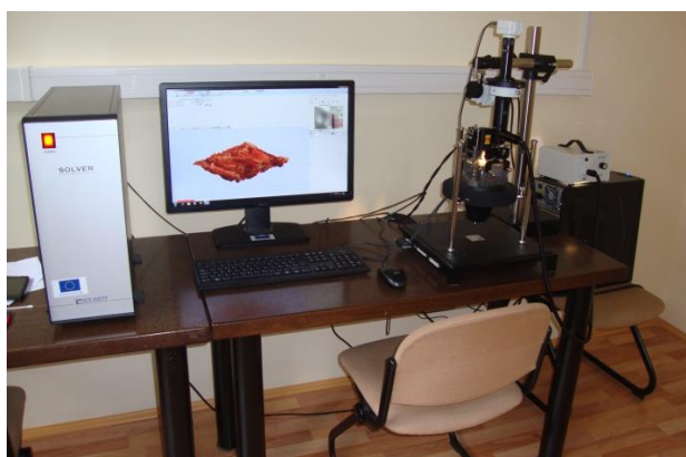
Fig. 3. NT-MDT Atomic Force Microscopy (AFM), at the Tribology Center on the Faculty of Engineering in Kragujevac.
