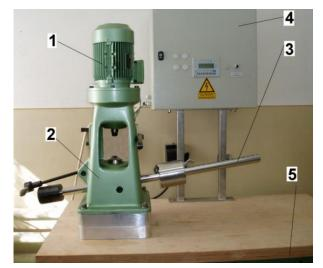
Fig. 1. The four ball machine.
