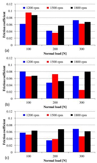
**Fig. 3.** Values of friction coefficient as a function of load and speed: (a) crude soybean oil, (b) degummed soybean oil and (c) transmission oil T90.
