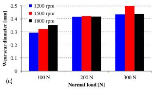
**Fig. 2.** Values of wear scar diameter as a function of load and speed: (a) crude soybean oil, (b) degummed soybean oil and (c) transmission oil T90.
