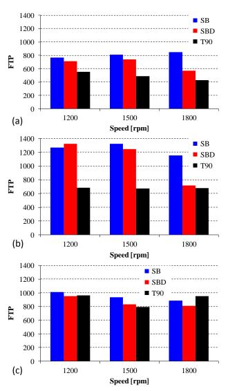
**Fig. 4.** FTP for the tested oils, for different rotational speeds and load: (a) 100 N, (b) 200 N and (c) 300 N.
