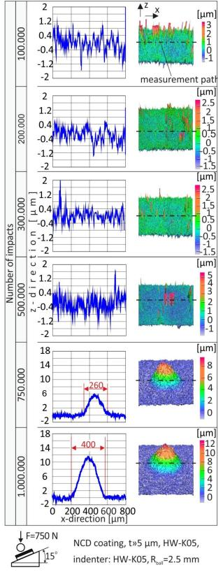
**Fig. 3.** Impact test results at an impact load of 750 N after various numbers of impacts.
