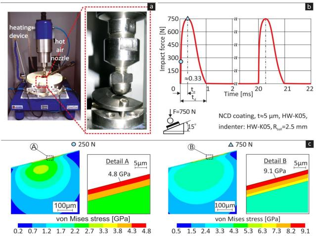
**Fig. 1.** (a) the mechanical unit of the employed impact tester, (b) characteristic data of the applied force signals and (c) the developed von Mises stress fields in the coating and its substrate during the inclined impact test.
