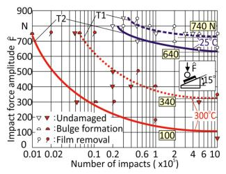
**Fig. 11.** Impact test results at various loads and temperatures for different film adhesion qualities.
