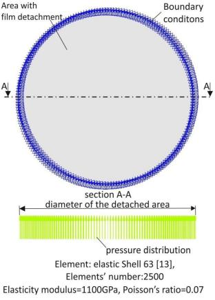
**Fig. 7.** Simulation of a coating bulge geometry by elastic shell elements.
