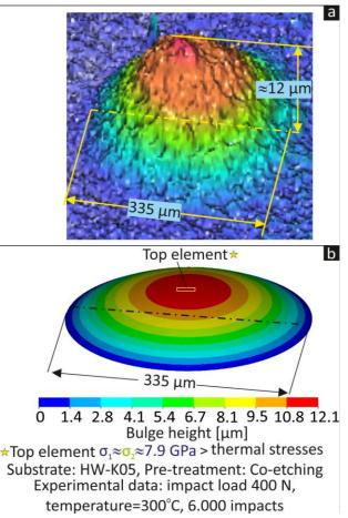
**Fig. 9.** (a) film bulge geometry after inclined impact test on NCD film on a substrate treated by Co-etching and (b) FEM calculated residual stresses for achieving the same bulge geometry.
