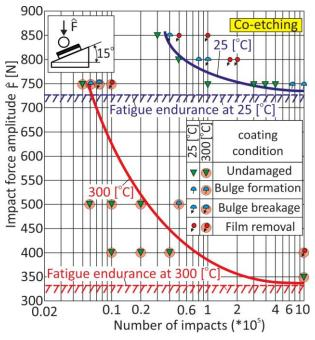
**Fig. 4.** NCD coating conditions after inclined impact tests with Co-etching substrate treatment.
