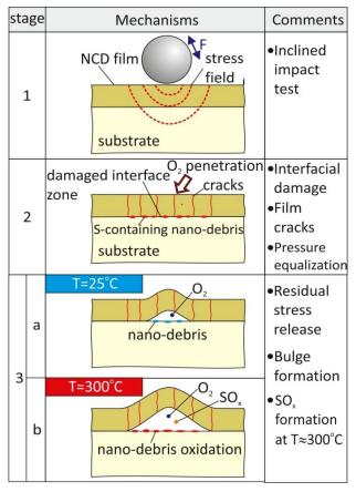
**Fig. 10.** Schematically presented mechanisms leading to diverse dimensions of NCD film bulges at various temperatures.
