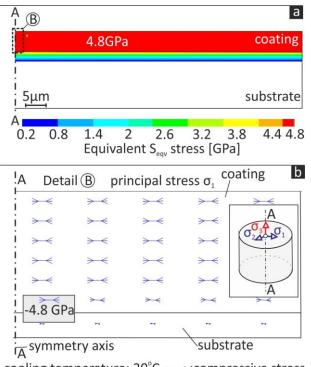
cooling temperature:  $20^{\circ}C \rightarrow \ll$  :compressive stress **Fig. 5.** (a) the developed equivalent stress field after cooling from the deposition temperature to the ambient one and (b) the relevant principal stress  $\sigma_1$  field.
