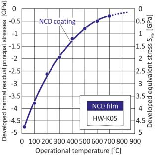
**Fig. 6.** Effect of the operational temperature on the developed residual principal and equivalent stresses in the NCD coating.
