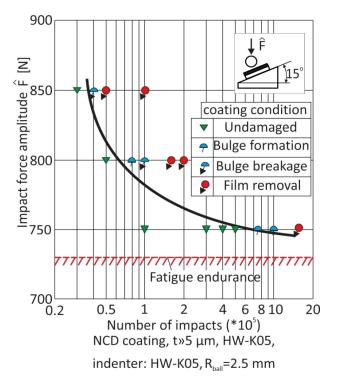
**Fig. 2.** NCD coating condition after the inclined impact test at various loads and numbers of impacts (Woehler-like diagram).
