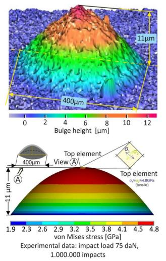
**Fig. 8.** Distribution of the measured displacement *z* and von Mises film stresses in the detached film region.
