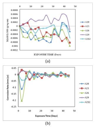
**Fig. 5.** Variation of (a) mass loss, and (b) corrosion rate with exposure time in 3.5 wt% NaCl solution for the Al-Mg-Si/75%Al<sub>2</sub>O<sub>3</sub>-25% RHA hybrid composites subjected different thermal cycles.
