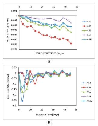
**Fig. 8.** Variation of (a) mass loss, and (b) corrosion rate with exposure time in 3.5 wt% NaCl solution for the Al-Mg-Si/RHA composites subjected to thermal cycling.
