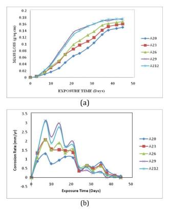
Fig. 11. Variation of (a) mass loss, and (b) corrosion rate with exposure time in  $0.3M H_2SO_4$  solution for the Al-Mg-Si/75%Al<sub>2</sub>O<sub>3</sub>-25%RHA composites subjected different thermal cycles.
