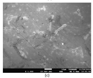
**Fig. 1.** Representative microstructures of the Al-Mg-Si based Composites containing 75 % alumina and 25 % RHA (A2) (a) no thermal cycling (A20), (b) after 6 thermal cycling (26), and (c) after 12 thermal cycling (A12).
