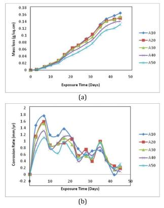
**Fig. 9.** Variation of (a) mass loss, and (b) corrosion rate with exposure time in  $0.3M H_2SO_4$  solution for the Al-Mg-Si/Al<sub>2</sub>O<sub>3</sub>-RHA composites which were not subjected to thermal cycling.
