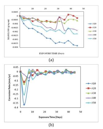
**Fig. 3.** Variation of (a) mass loss, and (b) corrosion rate with exposure time in 3.5 wt% NaCl solution for the Al-Mg-Si/Al<sub>2</sub>O<sub>3</sub>-RHA composites which were not subjected to thermal cycling.
