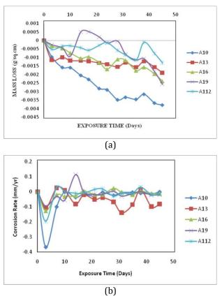
**Fig. 4.** Variation of (a) mass loss, and (b) corrosion rate with exposure time in 3.5 wt% NaCl solution for the  $Al/Al_2O_3$  composites subjected different thermal cycles.
