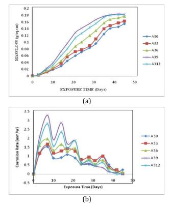
Fig. 12. Variation of (a) mass loss, and (b) corrosion rate with exposure time in  $0.3M H_2SO_4$  solution for the Al-Mg-Si/50%Al<sub>2</sub>O<sub>3</sub>-50%RHA composites subjected different thermal cycles.
