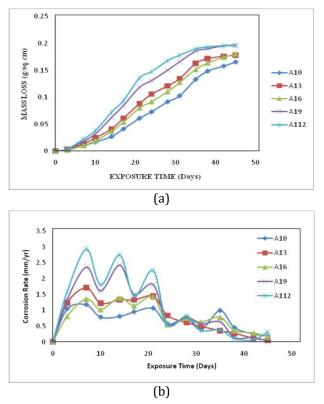
**Fig. 10.** Variation of (a) mass loss, and (b) corrosion rate with exposure time in  $0.3M H_2SO_4$  solution for the Al-Mg-Si/Al<sub>2</sub>O<sub>3</sub> composites subjected different thermal cycles.
