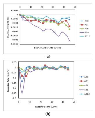
**Fig. 6.** Variation of (a) mass loss, and (b) corrosion rate with exposure time in 3.5 wt% NaCl solution for the Al-Mg-Si/50%Al<sub>2</sub>O<sub>3</sub>-50% RHA composites subjected to thermal cycling.
