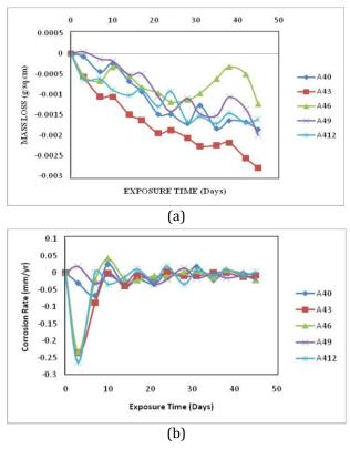
**Fig. 7.** Variation of (a) mass loss, and (b) corrosion rate with exposure time in 3.5wt% NaCl solution for the Al-Mg-Si/25 % Al<sub>2</sub>O<sub>3</sub>-75 % RHA composites subjected to thermal cycling.
