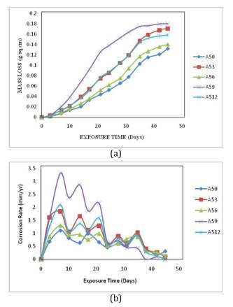
Fig. 14. Variation of (a) mass loss, and (b) corrosion rate with exposure time in 0.3M H<sub>2</sub>SO<sub>4</sub> solution for the Al-Mg-Si/RHA composites subjected different thermal cycles.
