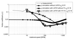
Fig. 7. Comparison of integral friction coefficients.
