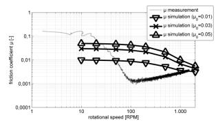
Fig. 4. Friction coefficients measurement and simulation.
