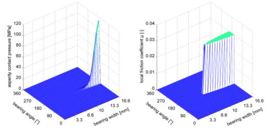
Fig. 5. Asperity contact pressure and constant friction coefficient.
