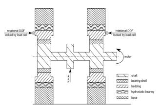
Fig. 1. Sectional view of plain bearing test bench.
