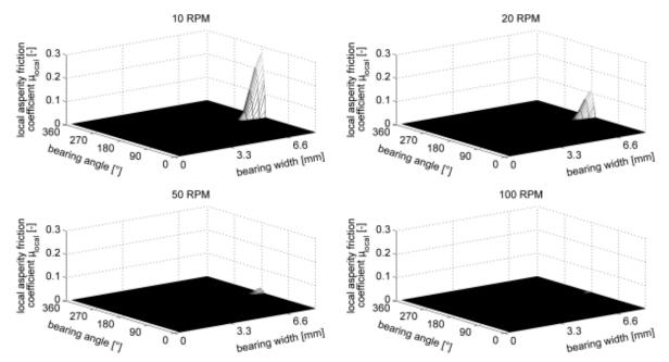
Fig. 8. Asperity friction coefficient at different rotational speed.
