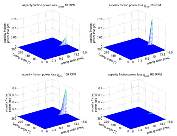
Fig. 10. Comparison of asperity friction power loss.
