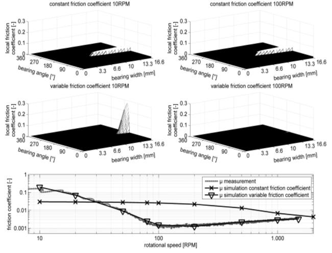
Fig. 9. Comparison of simulation results with and without local friction coefficients.
