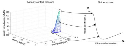
Fig. 6. Idea of locally dissolved friction coefficient.
