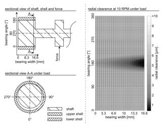
Fig. 3. Radial clearance under load at 10 RPM.
