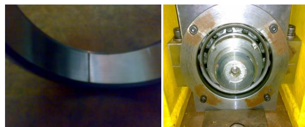
Fig. 5. Outer race seeded defect (0.5 mm width) & Test bearing housing.
