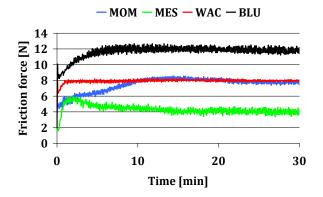
**Fig. 3.** Changes to the friction force in time for vulcanizates loaded with the force of 5 N.
