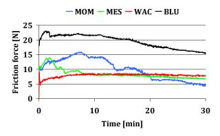
**Fig. 7.** Changes to the friction force in time for vulcanizates loaded with the force of 25 N.
