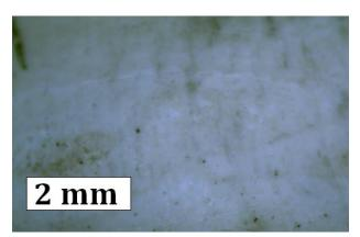
**Fig. 18.** The surface of MES vulcanizate after tribological test under the load of 30 N.
