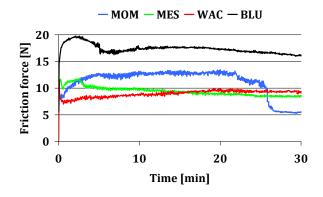
**Fig. 6.** Changes to the friction force in time for vulcanizates loaded with the force of 20 N.
