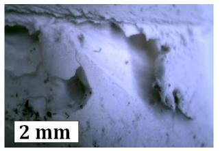
**Fig. 15.** Wear of the surface of MOM vulcanizate after tribological test under the load of 30 N.
