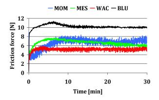
**Fig. 4.** Changes to the friction force in time for vulcanizates loaded with the force of 10 N.
