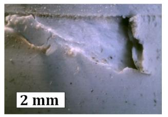
**Fig. 9.** Wear of the surface of MOM vulcanizate after tribological test under the load of 15 N.
