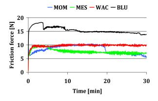
**Fig. 5.** Changes to the friction force in time for vulcanizates loaded with the force of 15 N.
