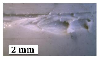
**Fig. 12.** Wear of the surface of BLU vulcanizate after tribological test under the load of 20 N.
