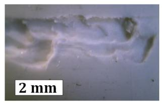
**Fig. 14.** Wear of the surface of BLU vulcanizate after tribological test under the load of 25 N.
