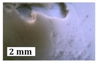
**Fig. 10.** Wear of the surface of BLU vulcanizate after tribological test under the load of 15 N.
