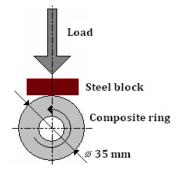
**Fig. 1.** Scheme of a block-on-ring contact applied in a T-05 tribo-tester.
