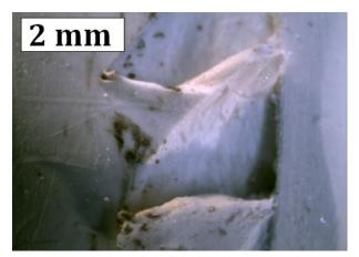
**Fig. 11.** Wear of the surface of MOM vulcanizate after tribological test under the load of 20 N.
