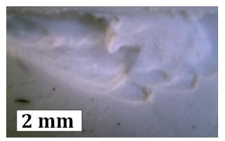
**Fig. 16.** Wear of the surface of BLU vulcanizate after tribological test under the load of 30 N.
