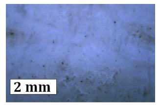
**Fig. 17.** The surface of WAC vulcanizate after tribological test under the load of 30 N.
