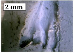
**Fig. 13.** Wear of the surface of MOM vulcanizate after tribological test under the load of 25 N.
