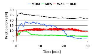
**Fig. 8.** Changes to the friction force in time for vulcanizates loaded with the force of 30 N.
