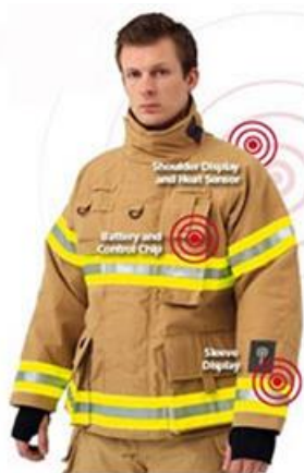
Figure 1. Intelligent fireman's outfit Four areas of innovation. Source: http://www.slipperybrick.com/2008/01/firefighters-sensor-jacket/
