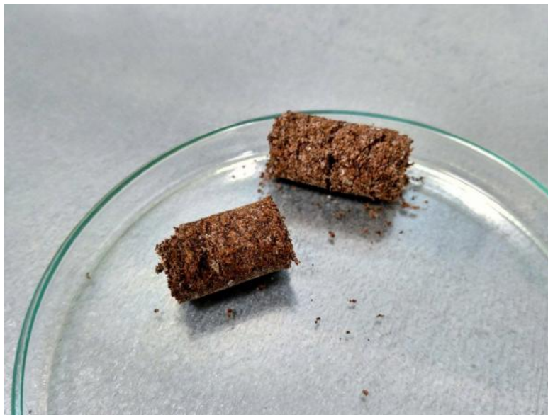
Fig. 2. Pellets made of black tea grounds with addition of starch as a binder Source: Author's
