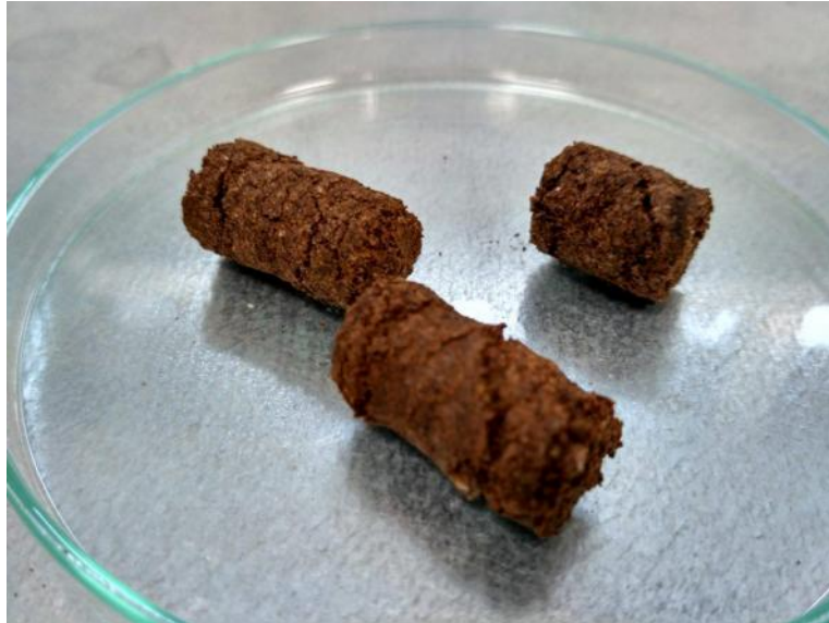
Fig. 1. Pellets made of coffee grounds with addition of starch as a binder Source: Author's
