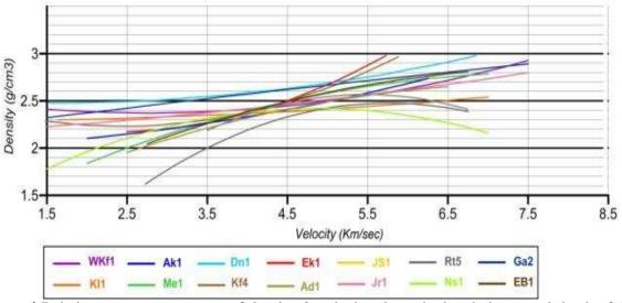
**Figure 4-**Relations curves to average of density & velocity along the borehole to total depth of (14) regional deep wells.
