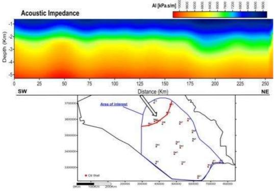
**Figure 13-**Showing the acoustic impedance profile model as a result of multiplying the scatter values of density by velocity, passing at the dip direction of the regional area (NE - SW).
