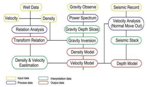
Figure 2-Flow chart of current geophysics integration based on (input data, processing, interpretation and output data).
