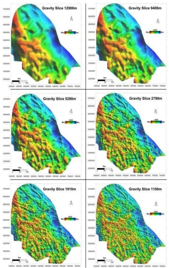
Figure 10-Showing the domination of grid levels interference in gravity domain, after applying the power spectrum analysis.
