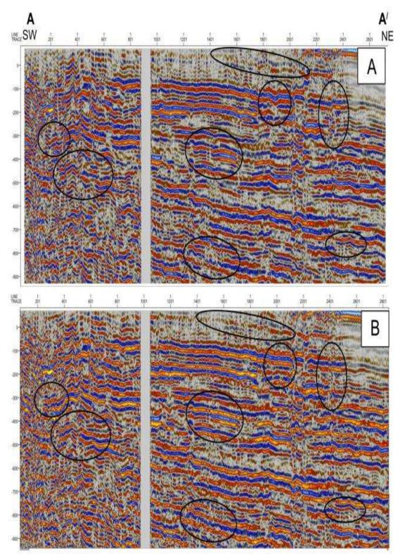
**Figure 18-**Shows seismic lines (7Gn- 16) compare it the results of seismic processing by apply the RMS (Present A) and by apply average velocity estimated from the gravity survey (Present B), the general enhancement reflectors foxed in black polygon.
