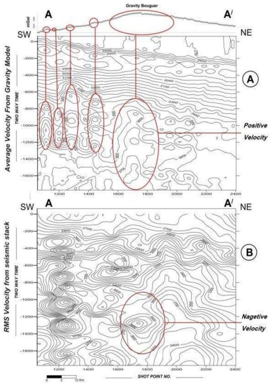
**Figure 16-**Compare the velocity model at seismic line between the average velocity estimated from gravity survey and RMS seismic processing velocity, shows the effective of big & small elements of gravity anomaly reflects positive velocity.
