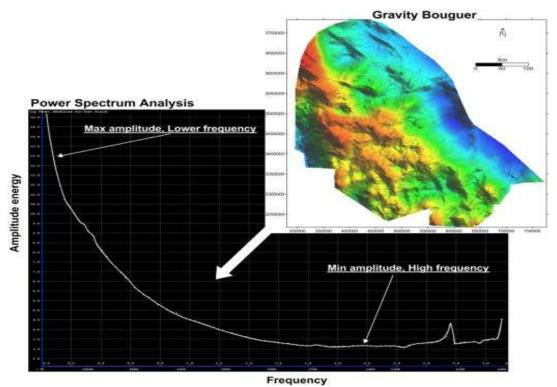
Figure 8-Power spectrum analysis of the gravity Bouguer, shows the spectrum of high to low amplitude and frequency.
