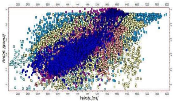
**Figure 3-**Function windows showing the scatter values of density & velocity relation along the borehole to total depth of (14) regional deep wells.
