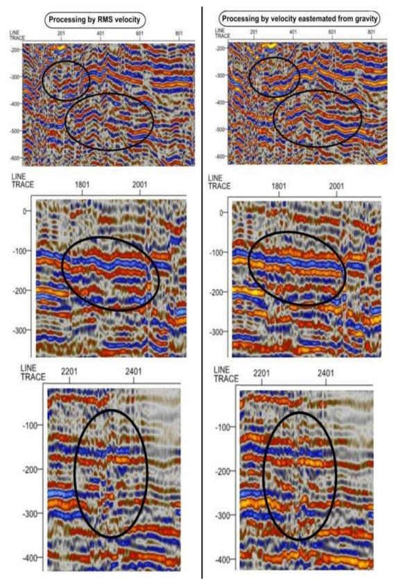
**Figure 19-**Shows the clear enhancement in improved seismic signal recorded that effective by the fault & fractures diffraction within seismic line (7Gn- 16) after applying average velocity estimated from the gravity survey.
