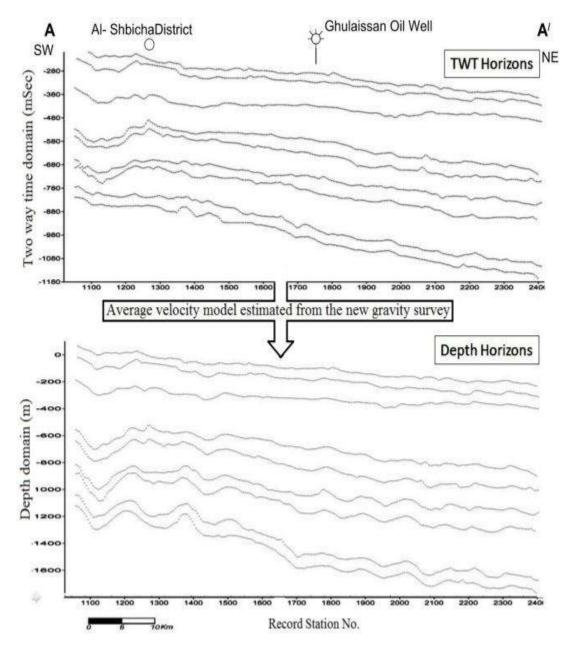
**Figure 21-**Conversion the time horizons from time to depth domains by average velocity model estimated from the gravity survey, shows the top formation surface kept its behaviors in depth domains indicating the logical velocity model applied.
