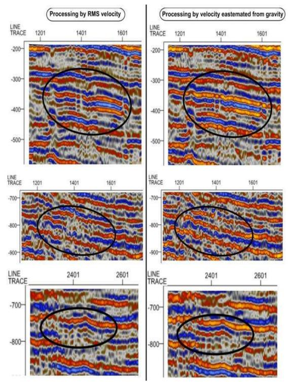
**Figure 20-**Shows the clear enhancement in improved seismic signal recorded that effective from the noise wave, by applying average velocity estimated from the gravity survey than applied RMS velocity, foxed within seismic line (7Gn-16).
