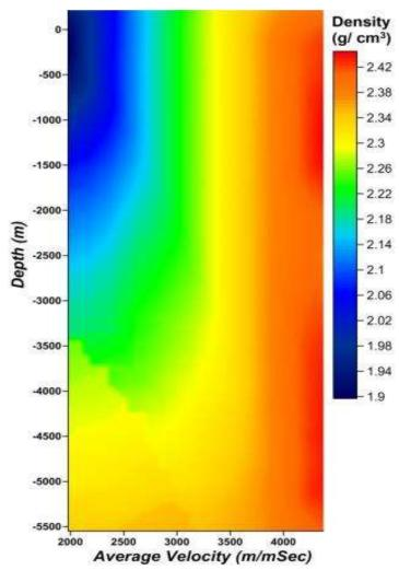
**Figure 7-**The density grid coverage from the scatter logs values in depth and velocity function of (24) wells in regional study area, shows the density behavior is divided into inhomogeneous distribution due to different environments laterally through depth levels.
