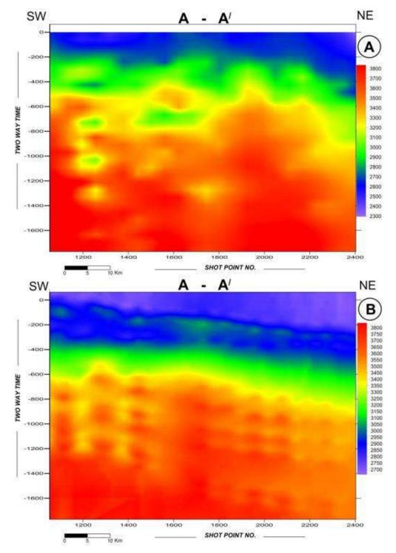
**Figure 17-**Compare the velocity distribution grid at seismic line (7Gn-16) between (A) RMS seismic processing velocity and (B) average velocity estimated from gravity survey. (B) Carries better stratigraphy means and obtains reverse velocity in shallowest level.
