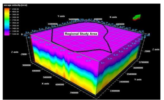
**Figure 15-**Showing 3D velocity cube (as segy format) in depth domain designed by conversion the 3D geometrical model to the velocity inverted from the gravity spectral slices.
