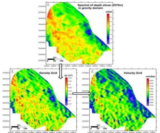
**Figure 12-** Showing the gravity inversion applying in 2D grid that biuld from (FFT Transform) to the profiles values of spectral depth slices in gravity domain to density and velocity domain.
