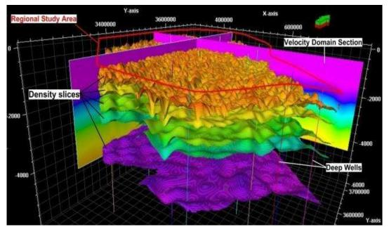
**Figure 14-**3D grid model in depth domain including the density surfaces slices through the section crossing of velocity model at the regional area of interest in central Iraq. Relatively the density of sediments increases with depth but density contrast decreases with depth,[12].
