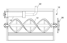
**Figure 2.** Speedy Dryer 10: Main Dody, 10: Steam Jacket, 12: Mixer, 14: Dust Ereaser, 20: Heat Transformer, 22: Inner Gas Stream Line, 26: Rotator)
