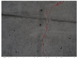
Fig16. a detection result image I from the distance of 5 meters
