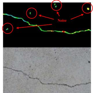
Fig3. A result of the detection method by the probabilistic relaxation method using line emphasis <sup>[9]</sup>
