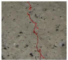
Fig14. a detection result image from the distance of 7 meters
