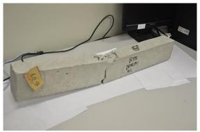
Fig7. Concrete crack specimen
