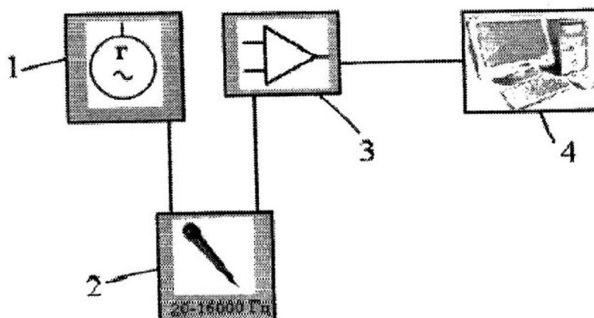
**Figure 1.** Block diagram of the device for the identification of the nerves of the larynx: 1 – alternator; 2 – sensor of sound signals (microphone); 3 – block of transformation of electric signals; 4 – block of processing of information and its display.
