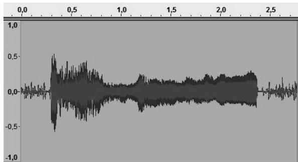
**Figure 5.** Signal at electrostimulation of wound tissues at a distance of 2–3 mm from the nerve.
