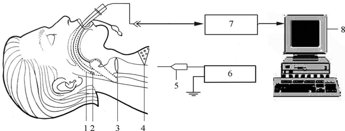
**Figure 2.** Technological scheme of identification of laryngeal nerves: 1 – laryngeal mask; 2 – sensor of sound signals; 3 – voice communication; 4 – surgical wound; 5 – electrode for irritation of wound tissues; 6 – alternator; 7 – filter and converter of sound signals; 8 – computer.
