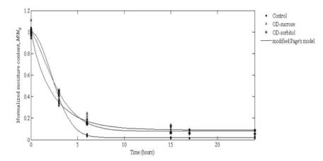
Figure 1. Experimental data and the fit of modified Page's model of the normalized moisture content (M/M0) during the freeze-drying of apple cubes
