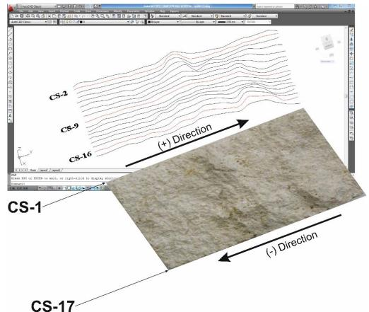
Figure 4. Rock Surface and Produced Cross-Sections
