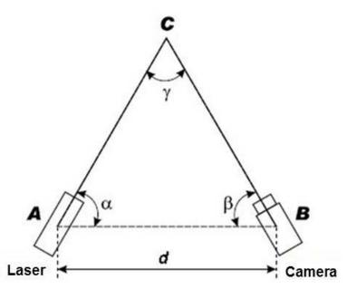
Figure 1Triangulation method in 3D Scanning.
