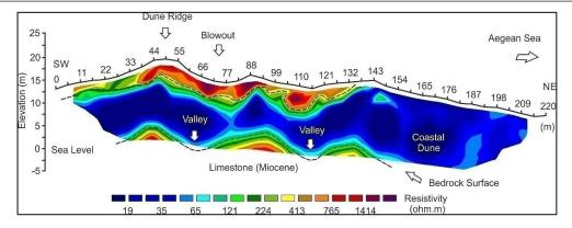
Figure 7. Electrical resistivity tomogram of surveyed line obtained from the inversion of apparent resistivity data.
