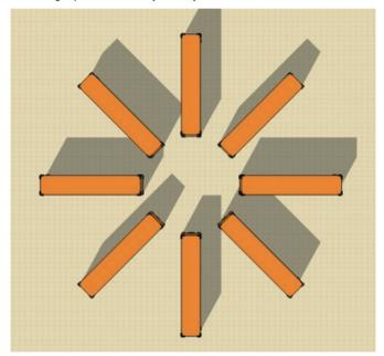
Each external element is covered with different materials, depending on its solar orientation. East and West orientations will have glass, South orientation maximizes solar energy capture through solar panels, and North is covered with ecologic insulation — cork. Rooftop gets protected with grass, abling water capture and filtration.
