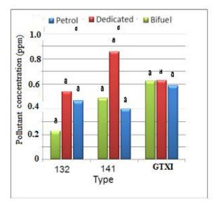
**Fig.2:** The amount of carbon monoxide production by different types of Pride with Petrol, dedicated, and bifuel fuel delivery systems (Mean data accompanied by different letters are significantly different according to Duncan's Multiple Range Test, p < 0.05) (*i.e.* a and a = not significantly different; a=maximum amount of pollutant production)
