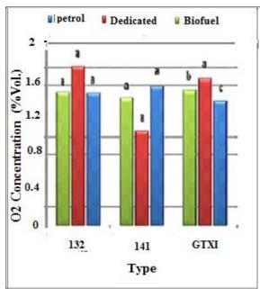
**Fig.4:** The amount of oxygen production by different types of Pride with Petrol, dedicated, and bifuel fuel delivery systems (Mean data accompanied by different letters are significantly different according to Duncan's Multiple Range Test, p<0.05) (*i.e.* a and b = significantly different; a and a = not significantly different; a=maximum amount of gas production)
