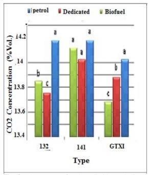
**Fig. 3:** The amount of carbon dioxide production by different types of Pride with Petrol, dedicated, and bifuel fuel delivery systems (Mean data accompanied by different letters are significantly different according to Duncan's Multiple Range Test, p<0.05) (*i.e.* a and b = significantly different; a and a = not significantly different; a=maximum amount of pollutant production)
