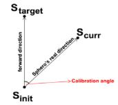
Figure 17. Calibration algorithm representation
