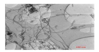
Fig. 2: TEM of Multi Walled Carbon Nanotubes.
