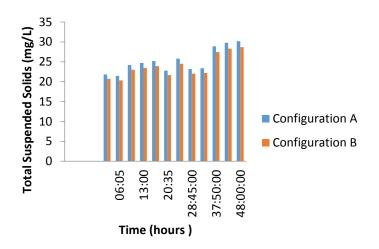
Figure 8: Relationship between TSS effluent quality and Hydraulic residence time
