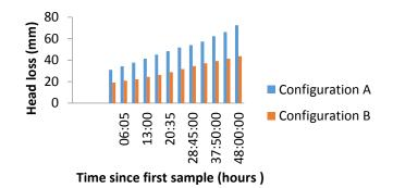
Figure 13: Relationship between Head loss and hydraulic residence time
