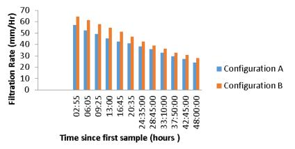
Figure 12: Relationship between Filtration rate and hydraulic residence time
