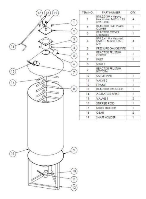
Figure 2: Exploded view of the Reactor
