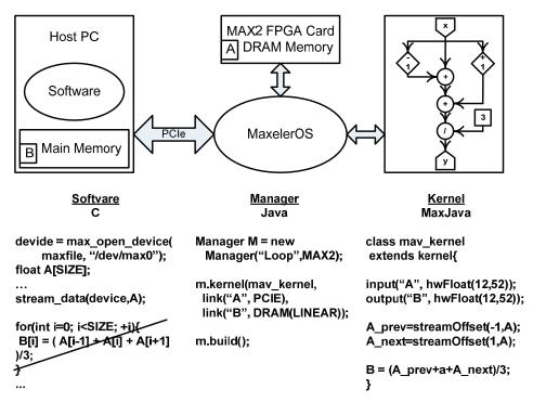
Fig. 3. Hardware/Software Relationship in a Maxeler DataFlow System.
