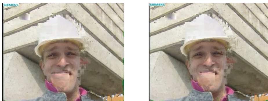
Fig. 4. The frames 34 (left) and 35 (right) of decoded protected video sequence streamed in a wireless environment with 2% of dropped packets.
