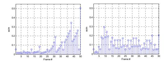
Fig. 5. SSIM indices of extracted watermarks from video encoded by an IBBBBB structure (left) and IBPBPBP predictive structure (right).
