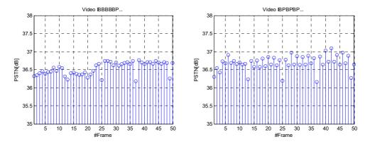
Fig. 4. PSNR for each frame of the decoded video sequence of an IBBBBBB structure (left) and an IBPBPBP structure (right).
