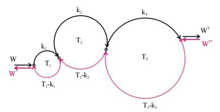
Fig. 1. An example of 3-stage Arnold transformation (solid line) and inverse Arnold transformation (dashed line) with the following parameters:  $k_1 = 8$   $T_1 = 24$ ,  $k_2 = 31$ ,  $T_2 = 48$  and  $k_3 = 12$ ,  $T_3 = 96$ .
