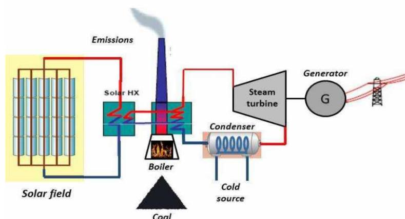
Fig. 2: Scheme of the integrated solar-thermal power plant.
