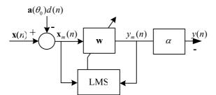
Figure 1. Block diagram of the proposed beamformer
