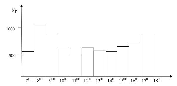
Figure 1. The diagram of distribution of passenger traffic flows on the bus route number 1
