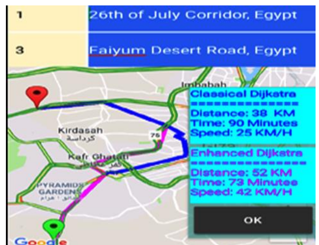
Figure. 5 The shortest route and the best route results between points 1 and 3 respectively
