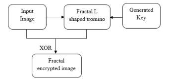
Figure.2 Fractal encryption stage
