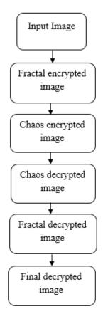
Figure.6 Block Diagram of Decryption Process
