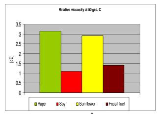
Fig. 3 - Relative Viscosity at 50<sup>o</sup>C of Bioliquids versus Liquid Fossil Fuel
