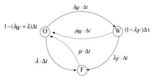
Fig. 1 The graph of state transitions of a used technical system
