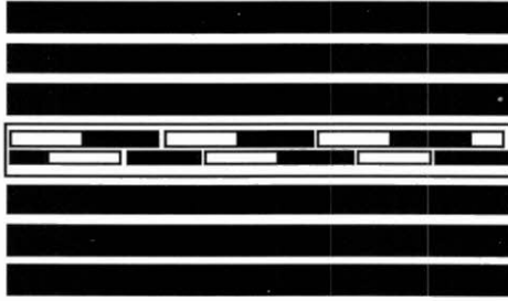
Gambar 2. Pola penyusunan venir bambu lamina Figure 2. Pattern of assembling laminated bamboo-veneer
