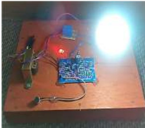
Fig.8 Basic circuit of clap switch
