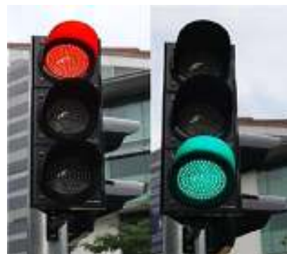
Fig. 9 Use of LED in traffic light Source: www.commonswikimedia.org
