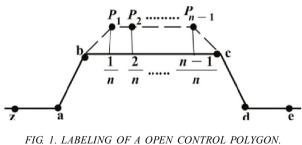
FIG. 1. LABELING OF A OPEN CONTROL POLYGON.  $p_{p}p_{2}...p_{n-1}$  ARE NEWLY INSERTED POINT BETWEEN OLD VERTICES b AND c
