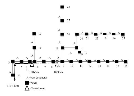
FIG. 2. SINGLE LINE DIAGRAM OF LVDN OF QUTAB FEROZAL, RAWILPINDI SUBDIVISION (PAKISTAN)
