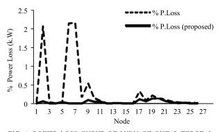
FIG. 4. POWER LOSS CURVE OF LVDN OF QUTAB FEROZAL, RAWILPINDI SUBDIVISION (PAKISTAN)
