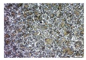
(a) OPTICAL (500X) (b) SEM(1000X) FIG. 5. MICROSTRUCTURE OF SPECIMEN B1 SOAKED FOR 1HRAT 8000C CONSISTS OF FERRITE (LIGHT) AND MARTENSITE (DARK)
