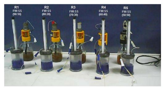
FIG. 1. REACTOR BOTTLES OF VARIOUS RATIOS OF FOOD WASTE AND SEWAGE SLUDGE ALONG WITH GAS MEASURING JARS
