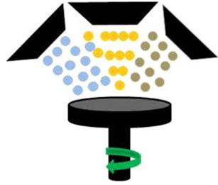
FIG. 1. SKETCH OF MAGNETRON SPUTTERING (WITH THREE MAGNETRONS TRAGETS). SAMPLE IS PLACED UNDER THESE TARGETS AND ROTATING WITH CONSTANT SPEED
