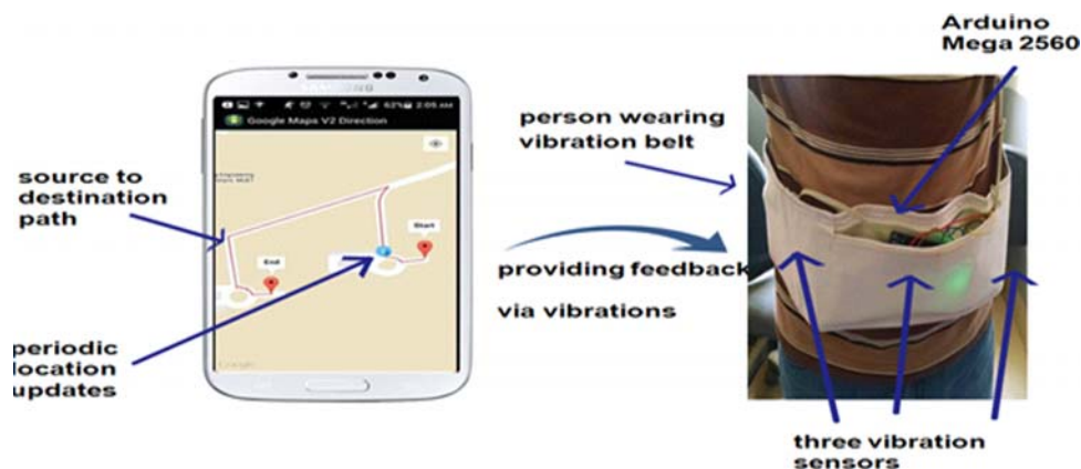
FIG. 4. APPLICATION PROVIDES DIRECTIONS FROM SOURCE TO DESTINATIONS VIA VIBRATIONS
