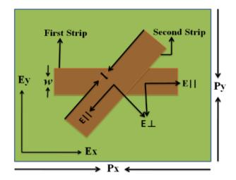
FIG. 2. SCHEMATIC UNIT CELL GEOMETRY OF DUAL LAYER POLARIZER
