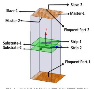
FIG. 4. A SAMPLE OF DUAL LAYER POLARIZER WHICH CONSISTS OF TWO PERIODICSTRIPS PRINTED ON BOTH SIDE OF INDIVIDUAL SUBSTRATE AND SEPARATED BY THE DISTANCE
