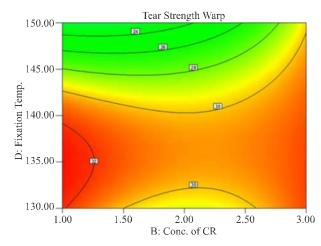
FIG. 8. CONTOUR PLOT OF CONCENTRATION OFCREASERESISTANT AND FIXATION TEMPERATURE
