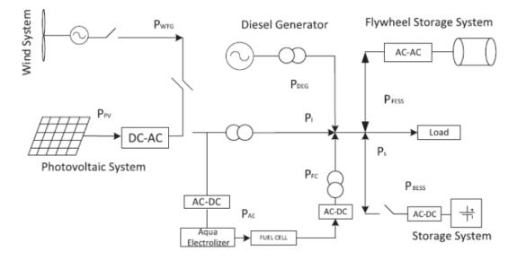
FIG. 2. STRUCTURE OF MICROGRID [6]
