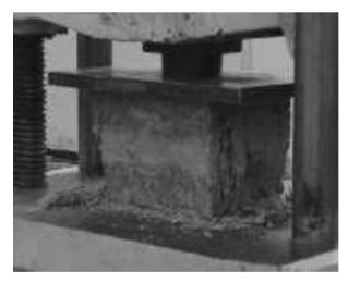
(c) TYPE-2, WITHOUT PLASTER FIG. 5. COMPRESSION TESTING OF MASONRY PRISMS
