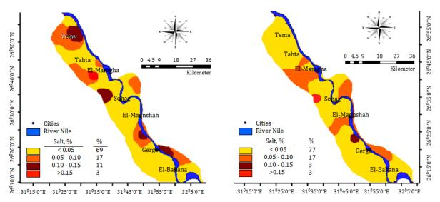
Figure 6. The changes in salt concentration of surface soil samples (0-25cm) irrigated by groundwater between 1991 and 2006.
