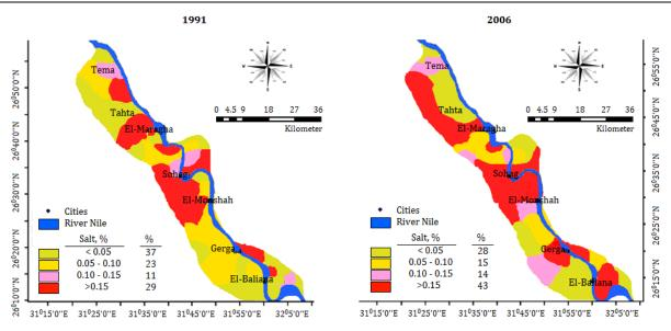
Figure 7. The changes in salt concentration of subsurface soil samples (25-50 cm) irrigated by groundwater between 1991 and 2006.
