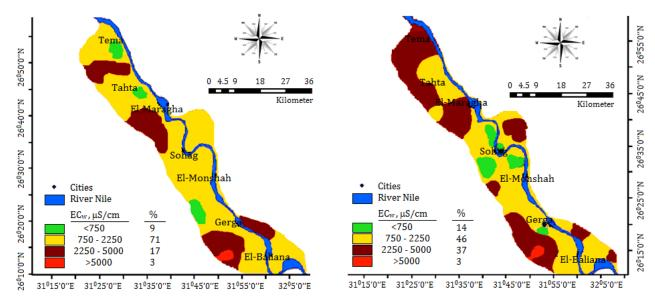
Figure 2. The changes in the electrical conductivity (EC<sub>w</sub>) of the groundwater between 1991and 2006.
