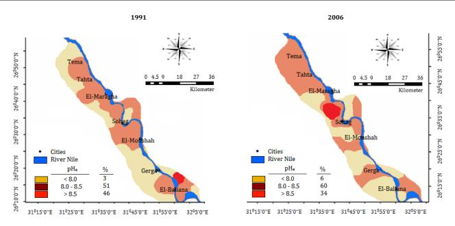
Figure 9. The changes in the pH of subsurface soil samples (25-50 cm) irrigated by groundwater between 1991 and 2006.
