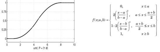
Figure 2. The S-Shaped membership function and its equation
