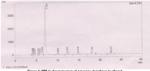
Figure 4: HPLC chromatogram of Artemisia absinthium in ethanol.
