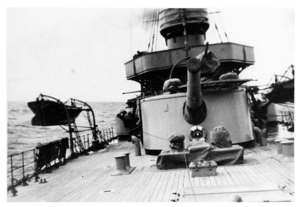
Fig. 3. The after 21 cm gunturret. The barrels of the after 57 mm guns are also visible
