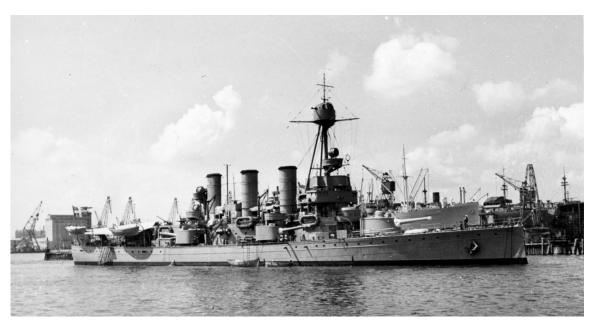
**Fig. 6.** «Oscar II» in Gothenburg 15 July 1946. A rangefinder is seen on her fighting top, life-floats are attached to the superstructure and the radio direction finder antenna has been moved to forward of the searchlight platform (photo is courtesy Curt S. Ohlsson)
